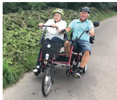
Figure 1. On the CwA, the pilot is placed behind the passenger(s) and only the pilot pedals. On the DB, pilot and passenger are next to each other and both are able to pedal. Photo to the left: Cycling without Age, June 8 2016. Photo to the right: Lassen, August 17, 2017.
