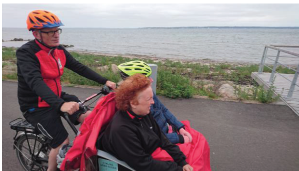
Figure 1. On the CwA, the pilot is placed behind the passenger(s) and only the pilot pedals. On the DB, pilot and passenger are next to each other and both are able to pedal. Photo to the left: Cycling without Age, June 8 2016. Photo to the right: Lassen, August 17, 2017.
