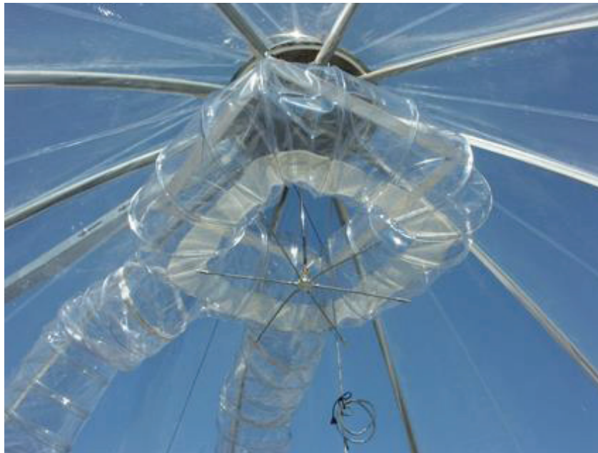
Figure 2. Interior of an ecotron mesocosm chamber showing equipment for controlling the circulation of atmospheric gases and humidity. Source: www.ecotron.cnrs.fr (accessed: 23.8.2016)
