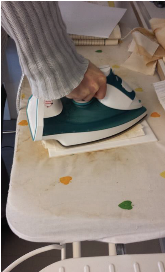
Figure 12. The transfer of laser-printer ink from glossy paper to copper laminated film. A ceramic tile can be spotted below the cloth protecting the glossy-paper-printed-circuit-film coupling (Photo: Alvise Mattozzi)
