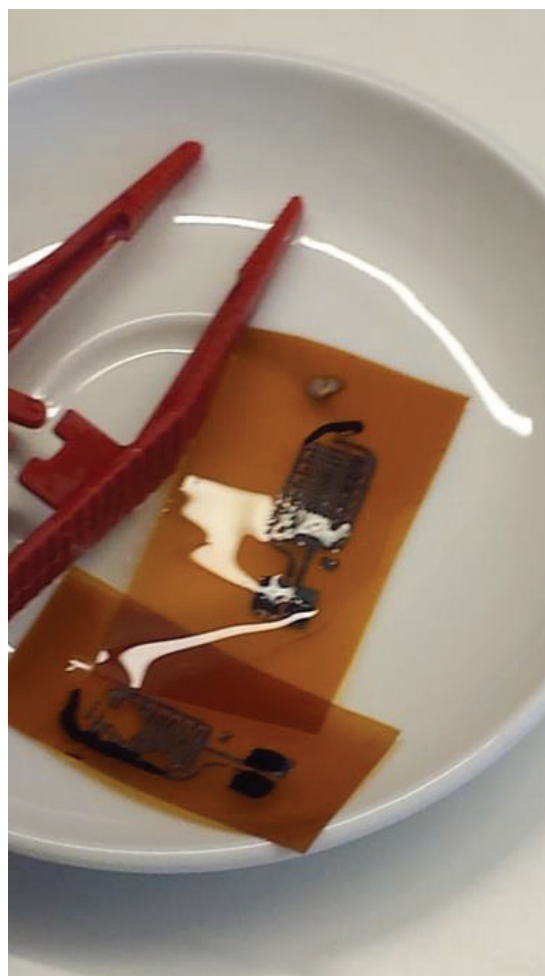
Figure 10. Circuits etched on copper laminated films (Photo: Alvise Mattozzi)
